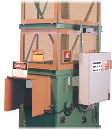
Roach custom-designed and engineered control panels may be ordered to Underwriters Laboratories UL® approval. Above electrical panel is painted optional Roach blue.
